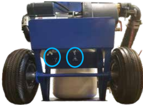
Figure 22: Remove wing nuts to remove pump from cart
