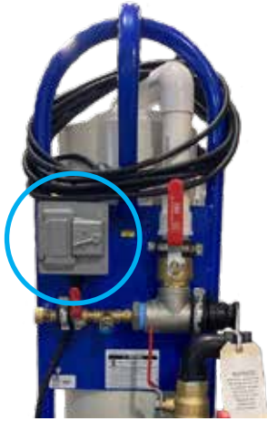
Figure 21: Remove electrical box from cart.
